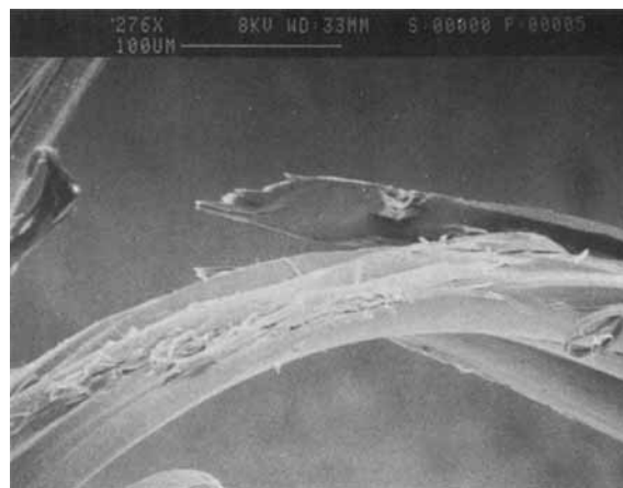
Figure 9 Higher magnification (275X) of fiber tensile sample in Figure 8.
